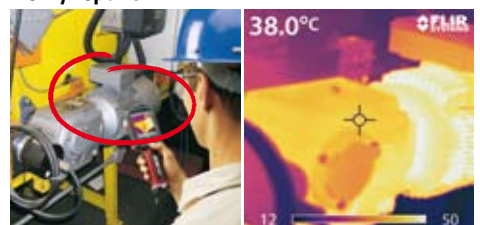
Mechanical check-up of an electrical motor using the FLIR i50.
